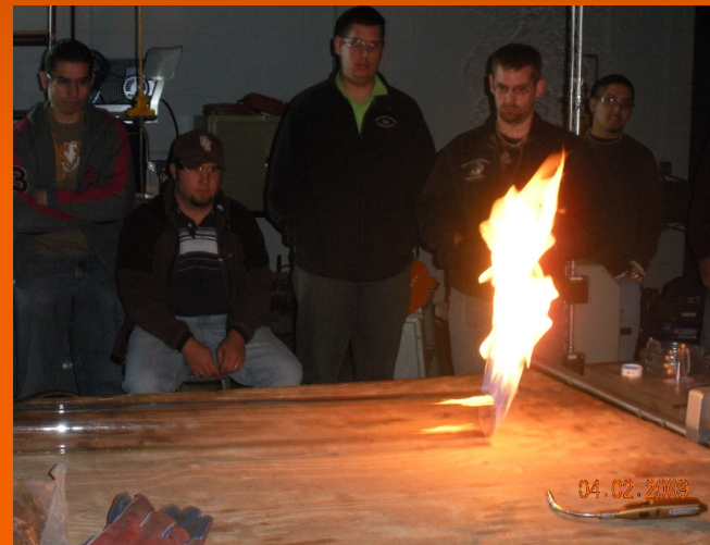
Fig.1 Lift-off occurs when the fuel flow is lean
