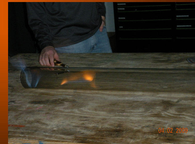
Fig. 3 Flame stabilization occurs when the flow of both propane and air is stoichiometric
